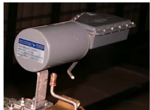
Figure 4b. New E-Glass Tube with Aluminum Label (Safe)
