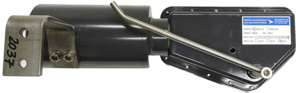
Fig. 4c. New E-Glass Tube with Aluminum Label (Safe)
