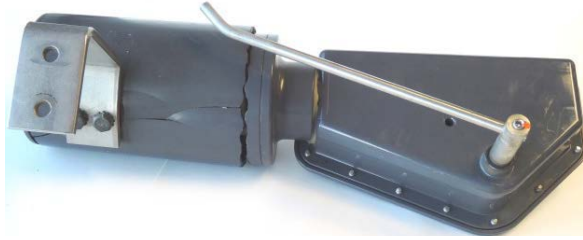
Figure 2. Fractured AmpVac Interrupter
