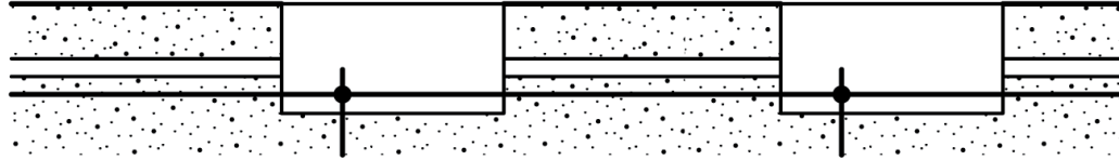
Figure 6.2. Direct buried conduits entering a series of vaults or handholes
