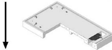
**Step 2.** Determine the height of vault needed, select any combination of 30-in **[B1]** or 48-in **[B2]** center sections (Stock Nos. 013131 and 013132, Section 6)
