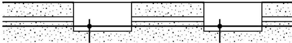
Install a continuous #2 AWG wire throughout the system and exothermically connect to the ground rod in each handhole. Route wire electrode in the bottom of the trench. Drill a hole into each vault wall for each grounding electrode entry. Drill each hole through the vault on the same wall that the conduits enter, above the water table if present. At entry into vault, exothermically weld each wire to eliminate air gaps between strands. Seal the wire's entry into vault to prevent water intrusion.
