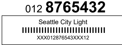
Figure 4.1.4a. Label with a 7-digit SCL Badge Number Embedded in the Serial Number (Not to Scale)
