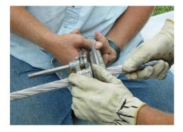
Located inside of the end fitting (steel forging) is an aluminum tube insert. The main purpose of this aluminum insert is to obtain a strong bond
