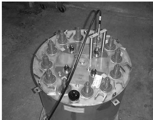
Figure 6. VACop IV Operator Attached to VACpac Switch.
