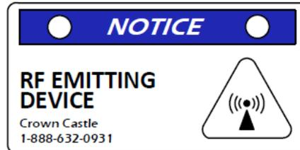
**Tag, RF Caution:** Where applicable, these tags are installed on small wireless facility and strand-mount antenna equipment enclosures and are clearly visible from the ground. This tag indicates that RF emissions may exceed the FCC Occupational Maximum Permissible Exposure (MPE) limits. See Figure 3g and SCL 0095.08.
