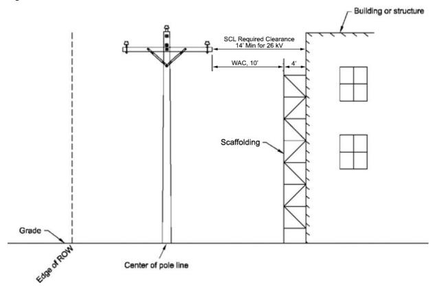
City Light transmission lines require even greater clearance. If a project requires work in proximity to any energized lines, we may de-energize and ground the lines, or relocate the lines temporarily. This work will be done at the customer's expense.
