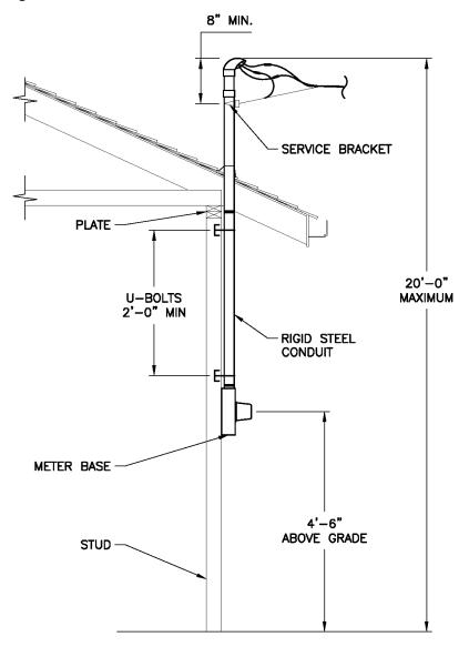
**WEATHERHEAD** SERVICE BRACKET MAST PLATE -RIGID STEEL CONDUIT U-BOLT NEAR PLATES EXTERIOR SIDING 20'-0" MAXIMUM U-BOLT MAY BE BOLTED TO STUD ON THE INSIDE FLUSH METER SOCKET METER BASE 4'-6" ABOVE GRADE
