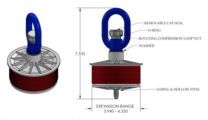
Figure 3.1c. 5-Inch Plug with Loop Nut, Stock No. 012389
