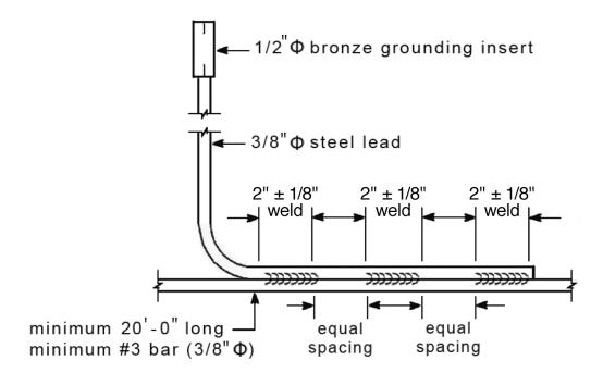
Each panel vault wall and floor shall be supplied with ground inserts.
