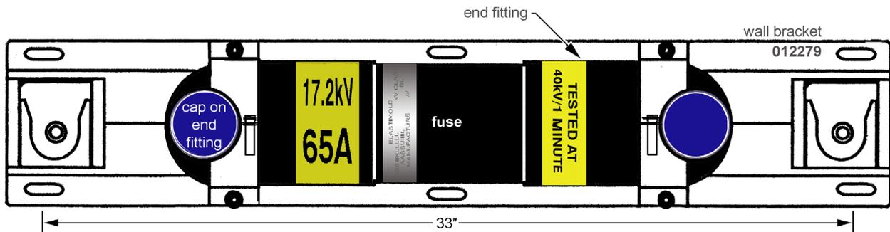
**Figure 4c. Molded Current Limiting Fuse with Tilt Mounting Adapter, Side View**
