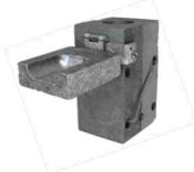
Molds shall have a minimum average life of 50 separate weld operations.
