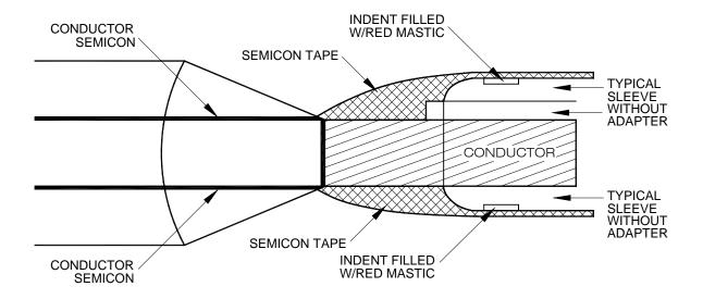
One or two half-lap layers of semicon tape over connector area.
