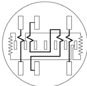
A Form 36S meter is a transformer rated 2 1/2 element meter used on the 26kV Feeder Survey. Unlike the 6S with 2 separate neutral blades, the 36S neutrals are tied to a common blade.
