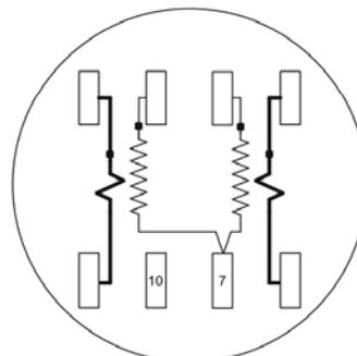
A Form 35S meter is a 2 element 3 wire transformer rated meter with a common potential return on blade 7.
