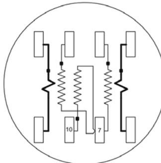
A Form 45S meter is a 2 element meter capable of 4 wire metering. When used on 3W installations, it is recommended that socket jaws 7 and 10 be jumpered at the socket or at the test switch. See pages 13, 15 and 21.
