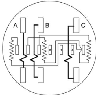
Form 9S meters are used on most of our 4 wire transformer rated services. When used on 4 wire Delta services, convention is to wire the high leg to C element. See page 21.
