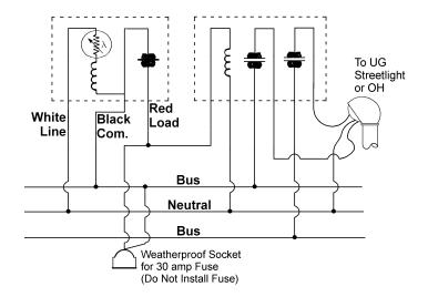
Flood Light Control Circuit with N.C. Streetlight Relay
