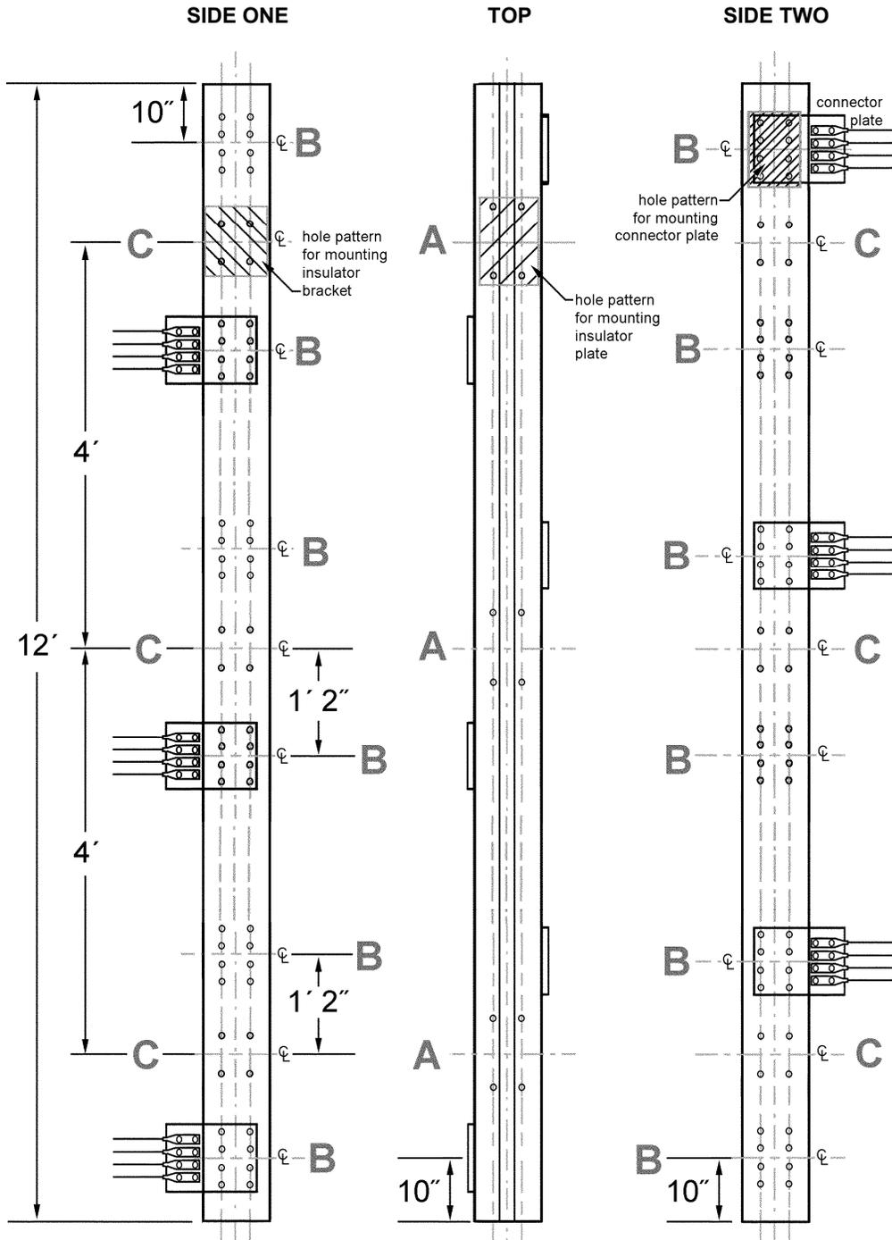
**A** = hole pattern centerline for mounting insulator plate, **top only** (item 20), separated by 2' 4" minimum, 8' maximum.
