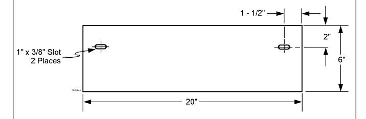
Tower/Circuit identification signs shall be of the configuration shown.
