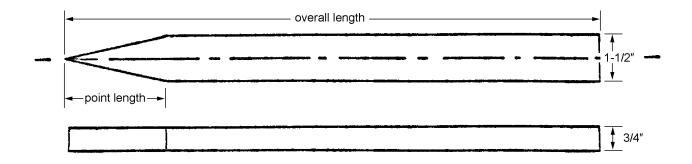
1. Survey Stakes shall be made from No. 1 select Western Redcedar or Douglas-fir. 1-1/2-inch sides shall be suitable for writing. Sound, tight 1-inch or smaller scattered knots are acceptable except in top of stake. Dimensions shall be as shown. Stakes shall have one end pointed to allow stake to be driven into the earth.
