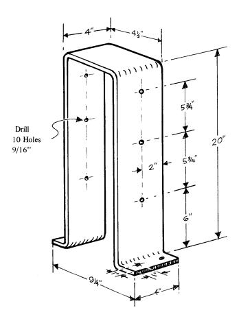
**Material:** Made from 3/8" x 4" flat, mild, hot-rolled steel. Galvanize after fabrication, in accordance
