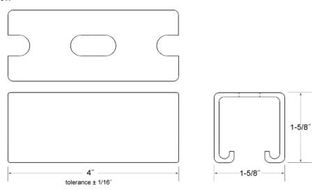
Cut channel on every-other slot (or hole) as shown. Grind ends and points smooth to eliminate hazard from sharp edges. Hot dip galvanize after cutting and grinding.
