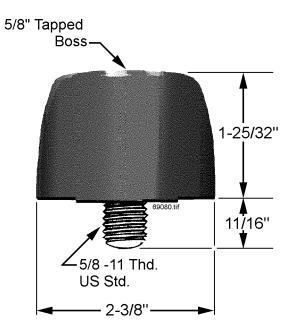
**General:** Molded phenolic insulator is intended for a maximum of 750 V service. All threads are 5/8" - 11 NC with a minimum of 11/16" thread depth. Cantilever rating is 250 foot pounds (minimum).
