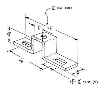
1. Material: Support shall be formed from 1/4" steel, electro-galvanized after forming, or may be any of the following standard 1-5/8" x 1-5/8" channel mounting brackets modified by increasing the diameter of the existing 9/16" center hole to 11/16" as shown.
