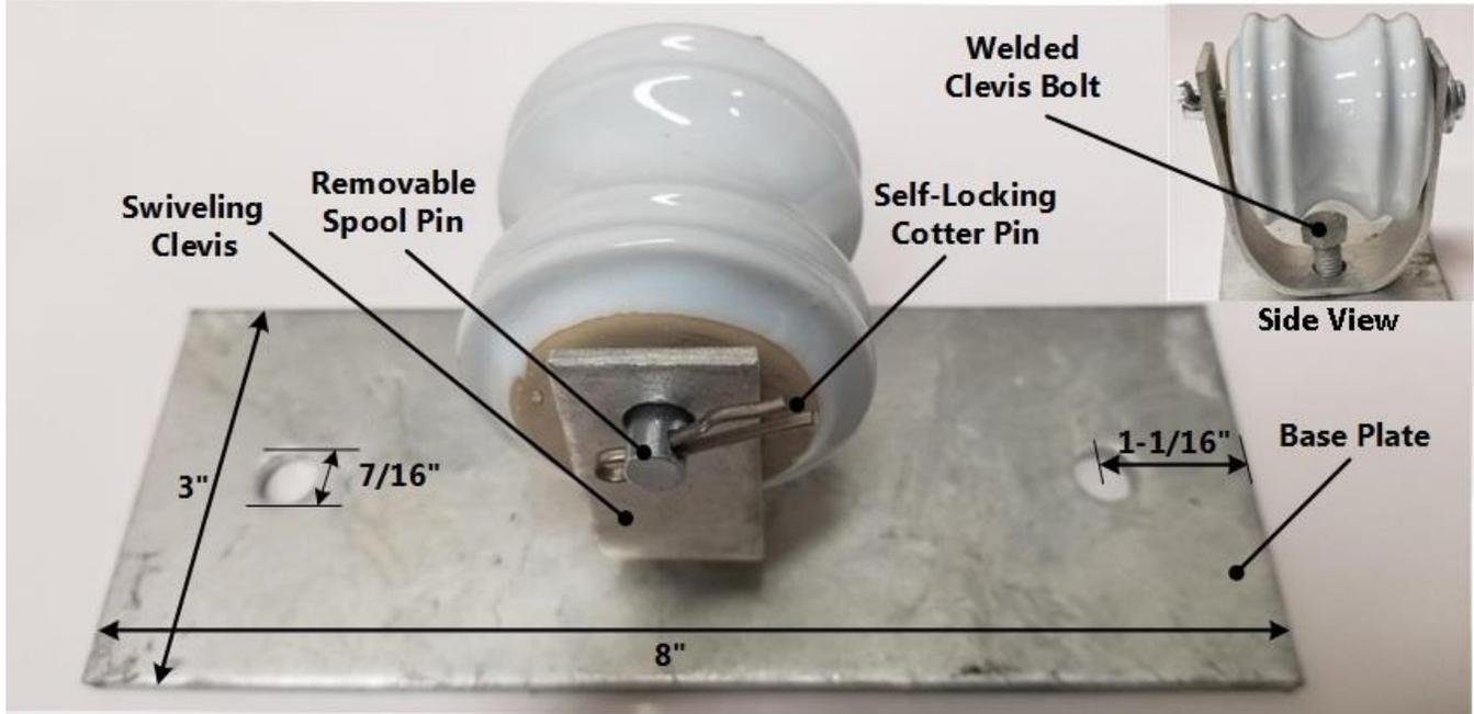
**Figure 4.2b. Roof-Mount Service Bracket**
