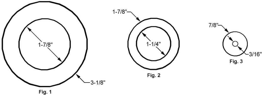
**Scope:** Silicone sponge rubber gaskets of the configurations shown are intended to be used on pole-type transformers where the gasket will be outdoors on a pole exposed to the sun, wind, rain, ozone, corona, and air pollutants.
