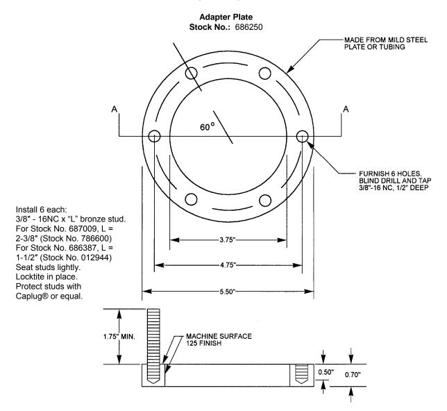
**Application:** For conversion of wiped lead pothead to straight 600 ampere bushing on 13 kV network transformers and other apparatus. See Stock Catalog page 70-47 for gasket and bushing Stock Numbers.
