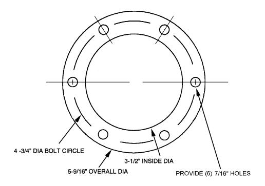
Material: Cork & Synthetic (Buna N) Rubber Composition: 3/16", C.L. Stock no.: 727687
