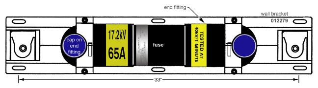
Figure 4c. Molded Curent Limiting Fuse with Tilt Mounting Adapter, Side View
