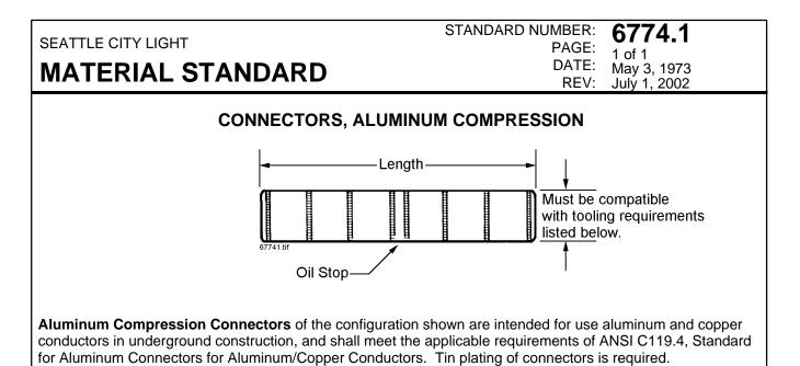
**Inhibitor**. Each connector shall be factory-filled with a measured amount of oxide-inhibiting compound that will not affect the dielectric strength or power factor of cables insulated with butyl, cross-linked polyethylene, or ethylene-propylene rubber.
