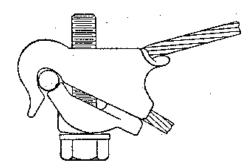
Aluminum Bolted Mid-Span Tap Clamps are used for making in-span taps on the neutral messenger of secondary aerial cable.
