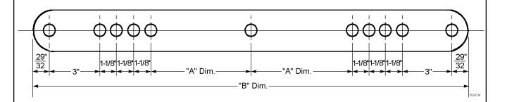
**Galvanized, Double and Quadruple Arming Plates** shall be 1/2" x 2-1/2" with 13/16" dia. holes. The plates are used for dead-ending, executing angles, and turning corners in overhead line construction.
