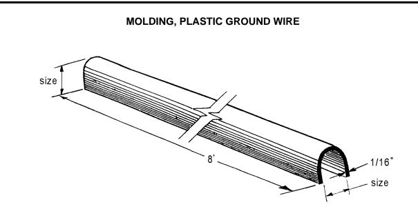
**Plastic ground wire molding** shall be made of a polyvinyl chloride compound which will not support combustion, have excellent weathering characteristics, remain stable and retain its uniformity in varying temperature ranges from 0° F to 110° F.
