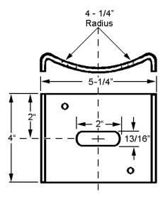
**Pole Gains** shall be of the configuration and dimensions shown and shall be of 3/16" carbon steel strip conforming to ASTM Specification A569.
