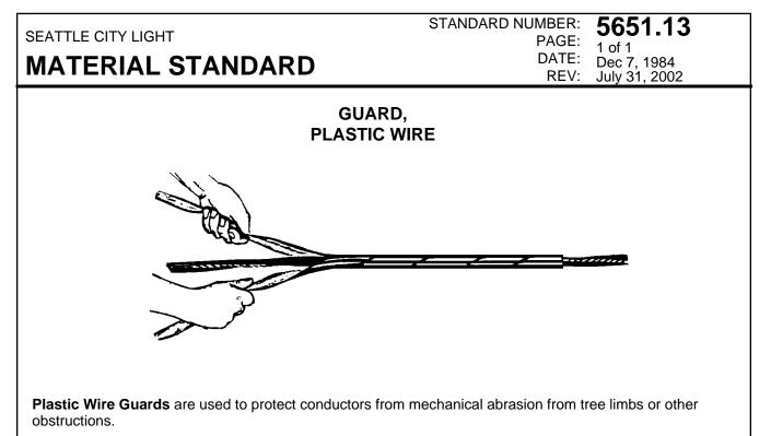
Wire guards shall be made of high-strength, high-impact, polyvinyl chloride thermoplastic compound that has good abrasion resistance, a low-moisture absorption rate, and excellent weathering ability.
