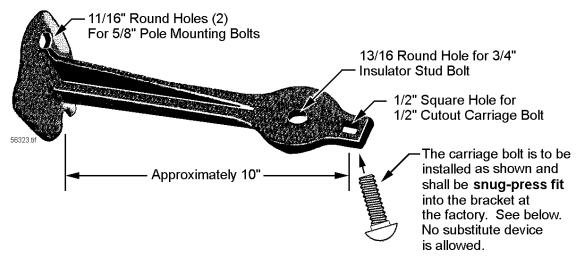
**Pole-Mounting Cutout Brackets**, of the configuration shown, are used to mount 26 kV open-type cutouts, with single 1/2-inch carriage bolt, directly to pole. The bracket shall be made of malleable iron conforming to ASTM A47, carbon steel conforming to ASTM A569, or ductile iron conforming to ASTM A536.
