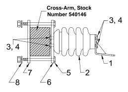
Note: Bracket is intended to secure station insulator (Stock No. 690187) to a 10 foot, 6 pin crossarm (Stock No. 540146).
