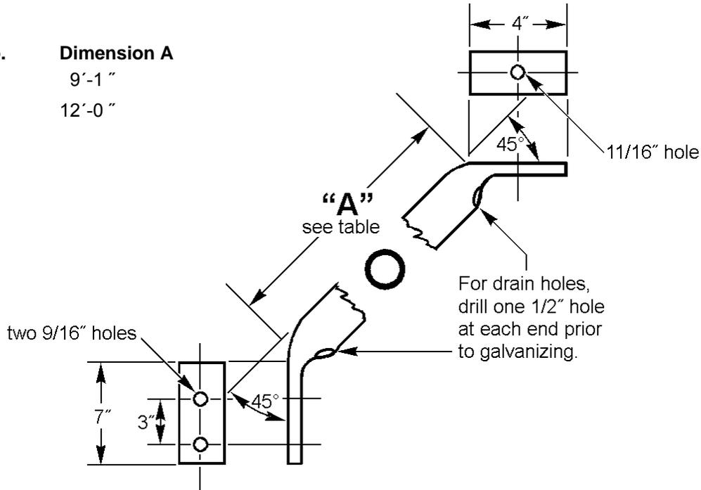
**9-Foot and 12-foot (nominal) Special Pipe Braces** shall be of the configuration and dimensions shown and shall be made of 1-1/4-inch, Schedule 40, standard black steel pipe conforming to the requirements of ASTM Specification A53.
