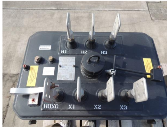
Figure 6.1b. Three-Phase Transformer Showing Location of the Terminals and Accessories
