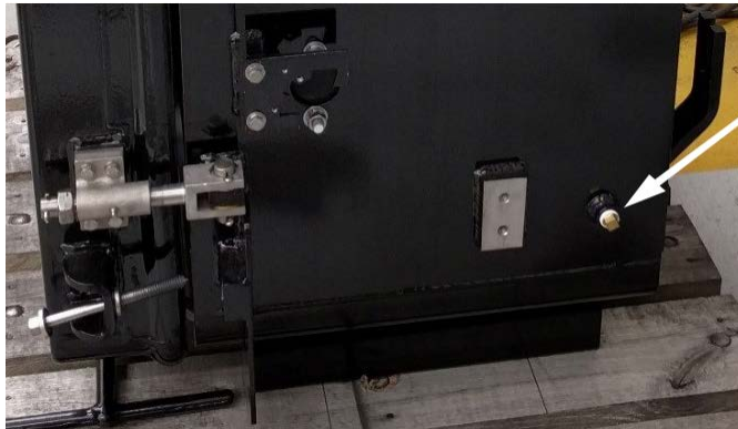
Figure 5.3a. Penetration on NP Right Hand Side for Remote Monitoring Equipment
