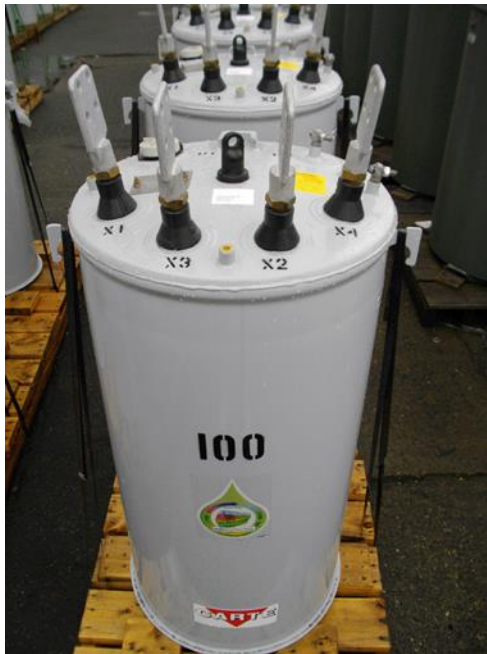
Figure 6.1. Transformer, showing location of the nameplate on the lid, kVA rating and fluid label
