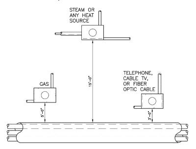
Figure 5.1b. Horizontal Clearances for Conduits and Duct Banks up to 26 kV, Water Structures, Plan View
