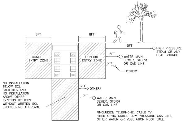
Note: If SCL conduit entry zones are planned for 115 kV or 230 kV, horizontal clearance shall be at least 5 fit between SCL conduit entry zones and non-SCL conduit or pipes.
