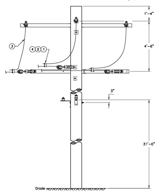
Figure 3m. Three-Phase Multi-Gain 0°-60° Tangent to Deadend 2 LPI Jumper, Top View
