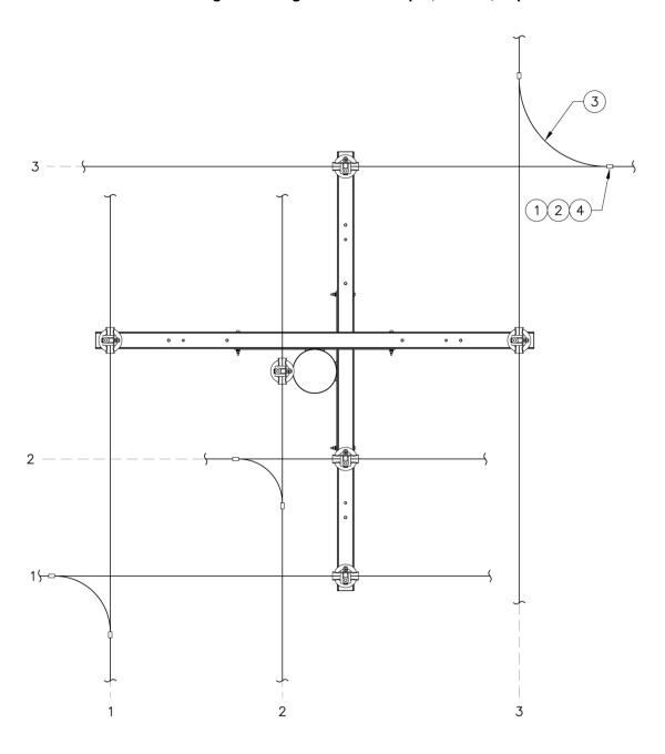
Figure 3v. Three-Phase Multi-Gain Tangent to Tangent No LPI Jumper, Alternate, Top View
