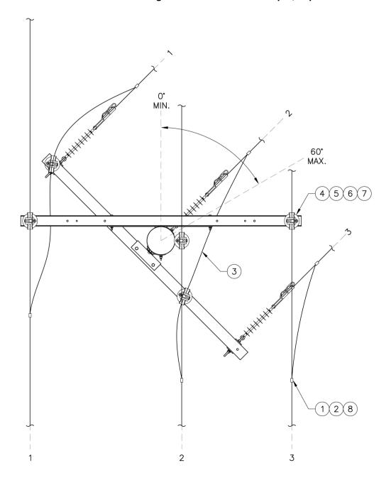
Figure 3n. Three-Phase Multi-Gain 0°-60° Tangent to Deadend 2 LPI Jumper, Side View
