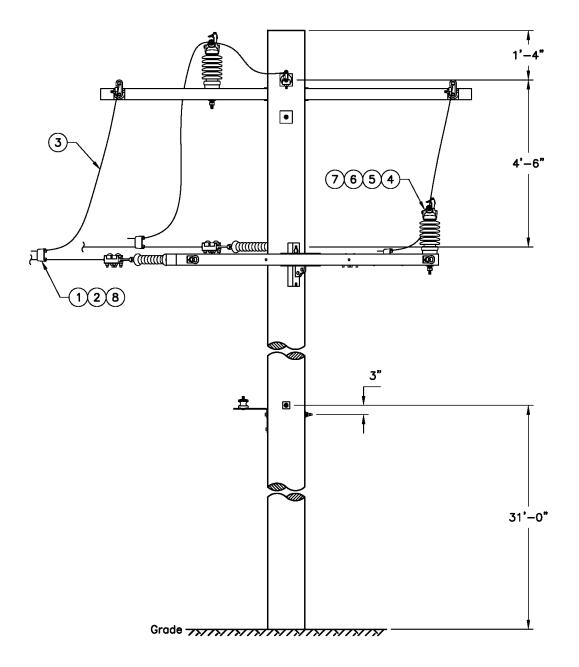
Figure 3g. Three-Phase Multi-Gain 60°-100° Deadend to Deadend 3 LPI Jumper, Normal, Top View
