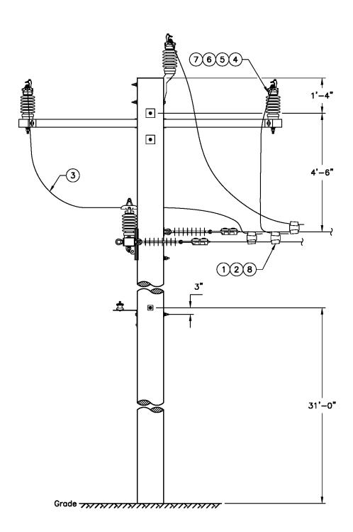
Figure 3s. Three Phase Multi-Gain 100°-180° Tangent to Deadend 2 LPI Jumper, Top View
