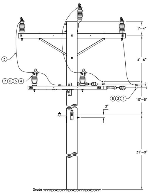
Figure 3o. Three-Phase Multi-Gain 60°-100° Tangent to Deadend 1 LPI Jumper, Normal, Top View
