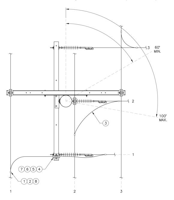
Figure 3p. Three-Phase Multi-Gain 60°-100° Tangent to Deadend 1 LPI Jumper, Normal, Side View
