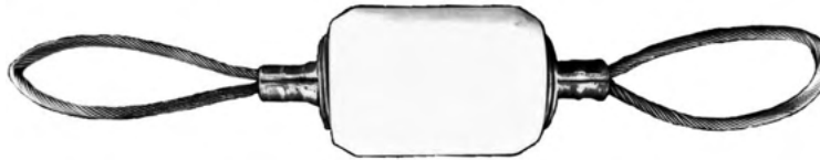
Figure 3a. Mandrel with Stainless Steel Cable
