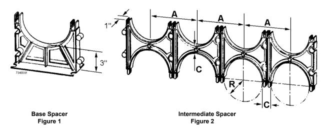
**Plastic Spacers for Nonmetallic Conduit** shall be of the general configuration shown, and shall be molded from a general-purpose polystyrene meeting the requirements of ASTM Standard D4549 for Type 1 molding material.
