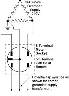
3Ø 3-Wire **POWER LOAD** (grounded at one corner)
