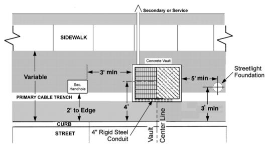
When vault or handhole extends into the sidewalk area because of a narrow planting strip, the vault or handhole shall be located entirely in the sidewalk with the edge flush with the street edge of the sidewalk and to the sidewalk grade. This applies only to the alternate location.
