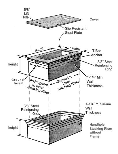
Type 1 and Type 2 Open Bottom Handhole, Precast, Secondary and Streetlight
