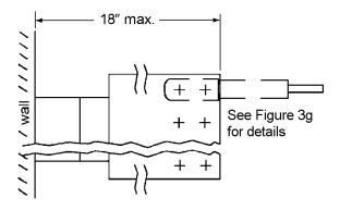
Figure 3.10c. Bus Bars Parallel to Floor, Elevation View (Cables Parallel to Floor)
