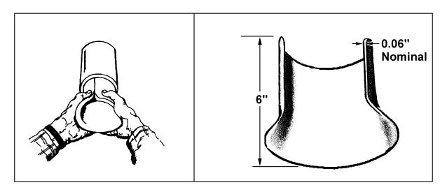
**Cable Protectors** for installation in duct and conduit ends shall be of the configuration shown, and shall be made from stress-relieved virgin nylon meeting the requirements of ASTM D789 or high-density polyethylene meeting the requirements of ASTM D1248. The material shall have the following additional requirements.
