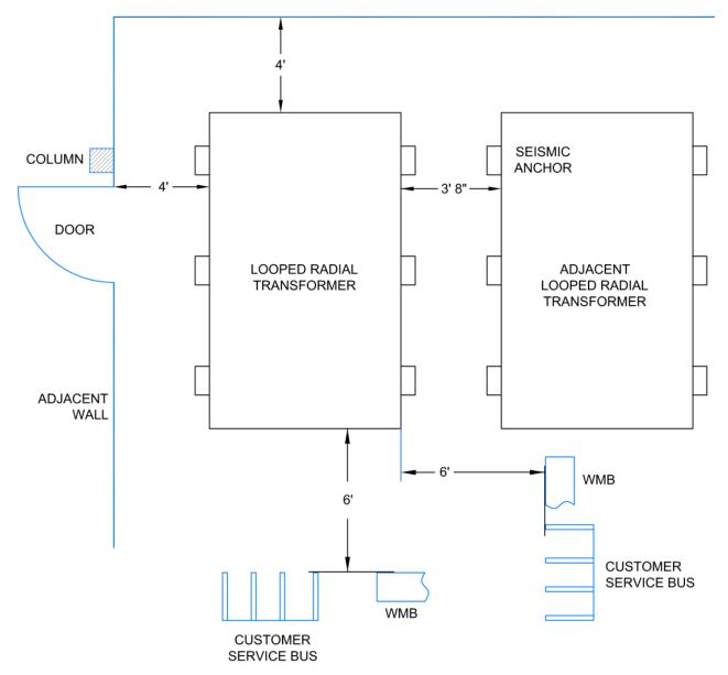
Figure 3.7c. Looped Radial Single-Phase Transformer Working Space, Plan View
