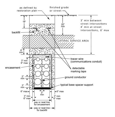
Figure 4.2. General Duct Bank, Side View
