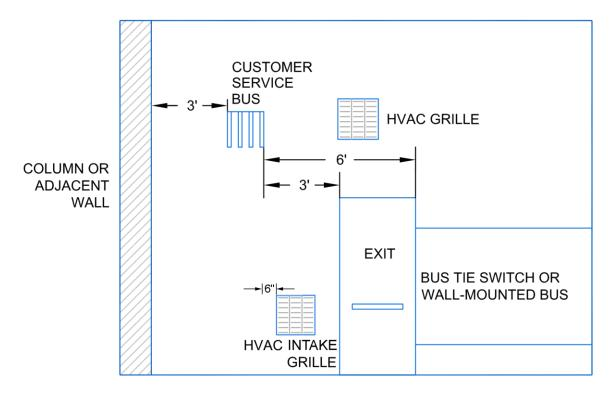
Note: HVAC grille clearance can be reduced for intake grilles per the figure above. See additional requirements in SCL 0751.00.
