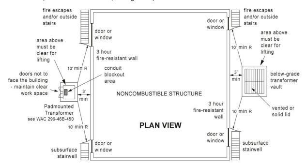
**Figure 9.1b.** Noncombustible Structures (Structures Designed to Resist Fire for Three Hours), elevation view (for combustible structures, see Figure 9.2)
