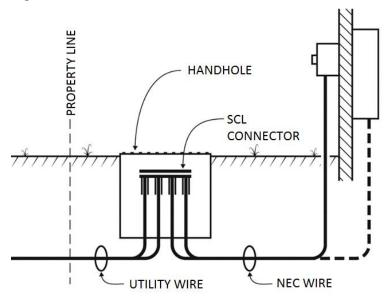
The minimum interior dimensions are based upon the number of cables entering the handhole. Table 5.4 shows required dimensions for service termination handholes.
