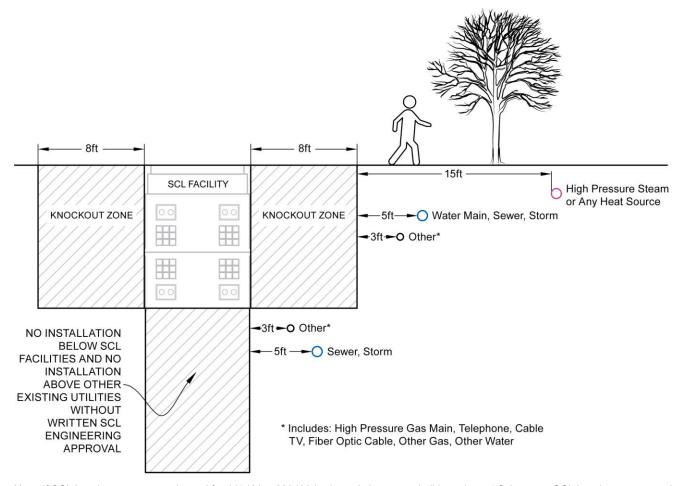
Note: If SCL knockout zones are planned for 115 kV or 230 kV, horizontal clearance shall be at least 5 fit between SCL knockout zones and non-SCL conduit or pipes.
