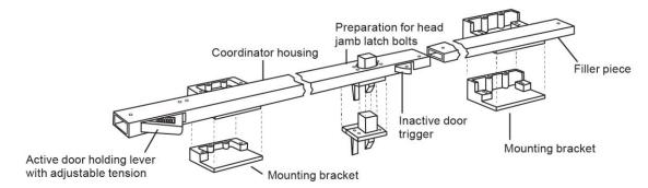
Coordinators shall be one of the following products or an equal approved by SCL prior to construction:
