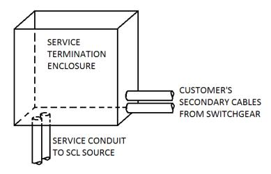
Conduits shall enter near the corners of the service termination enclosure but not through the back of the enclosure. Conduits shall not enter the same corner of the enclosure from two directions.
