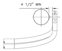
Figure 3.1d. Wraparound Steel Conduit Riser, Profile View
