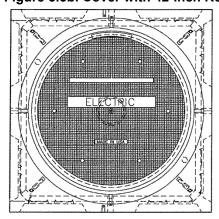
Figure 5.3c. Cover with H30 Hatch
