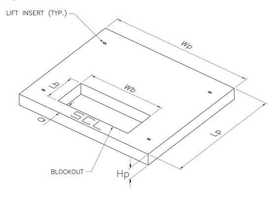
Precast Reinforced Concrete Transformer Pads
