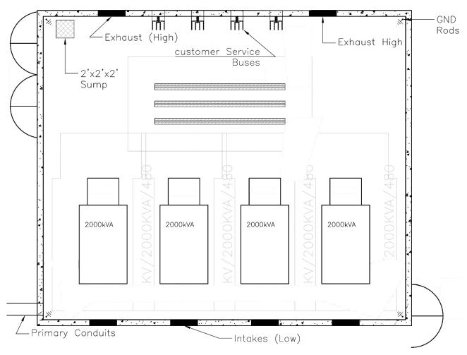
9.1 In-building vaults shall be dry spaces, and no standing water shall accumulate in the vault. The customer shall take adequate measures to prevent water from entering the inbuilding vault via wall, floor, or ceiling penetrations or via seepage. It is the responsibility of the customer to maintain the vault as a dry space.
