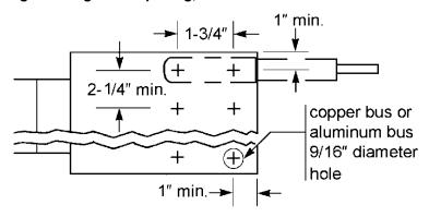
Figure 3.10h. Hole Spacing, Two-Hole Vertical Connection
