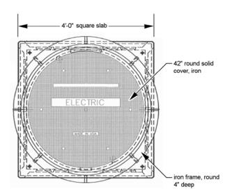
Figure 5.3c, Slab with 36- by 36-Inch Hatch (Stock Number 013157)
