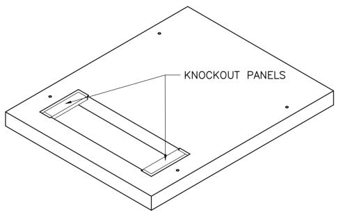
Lift inserts measuring 3/4-inch in diameter (nominal) shall be located at each corner on the top side of the pad.
